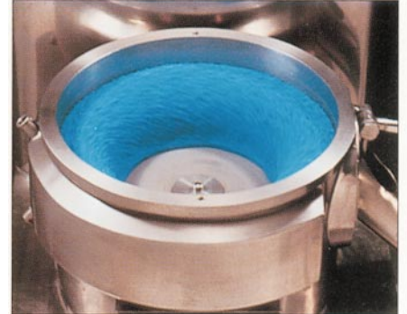
The Marumerizer™ transforms pellets into smooth, uniform spheres.
