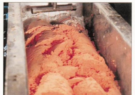
Mixers and kneaders provide the proper powder/liquid mixture for subsequent extrusion.
